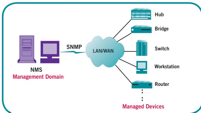
◀ **A typical scenario of a Network Management System (NMS) managing multiple devices over Local and Wide Area Networks.**
